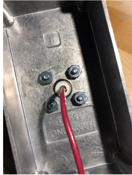
S0-239 chassis mount connector attached to the inside view of the aluminum enclosure
