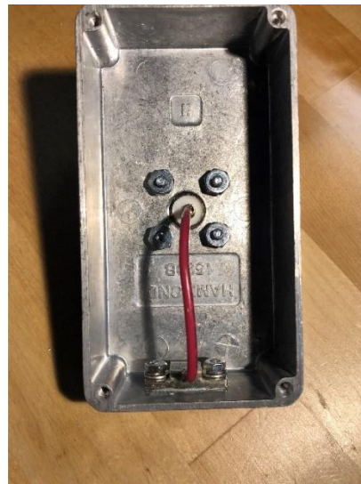
feed line from the S0-239 connector to the tab on the flange mount microwave termination resistor Figure 13
