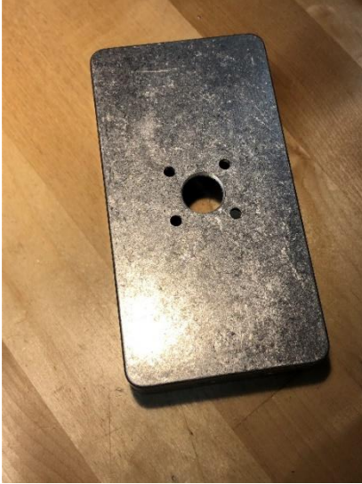
SO-239 4-hole chassis mount connector holes Figure 6
