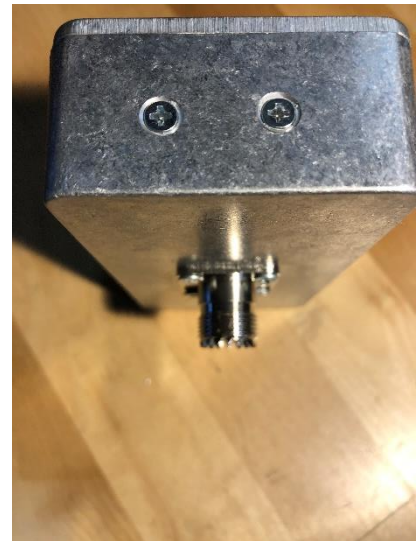
Enclosure end view resistor mounting screws
