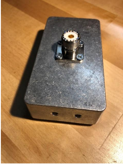
S0-239 chassis mount connector attached to the outside view of the aluminum enclosure
