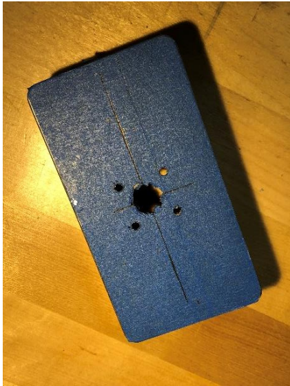
SO-239 4-hole chassis mount connector holes Figure 3
