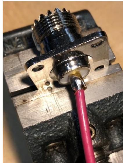
Feed line wire soldered in SO-239 connector solder cup Figure 9
