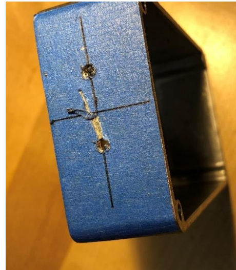
Flange resistor mounting holes Figure 4
