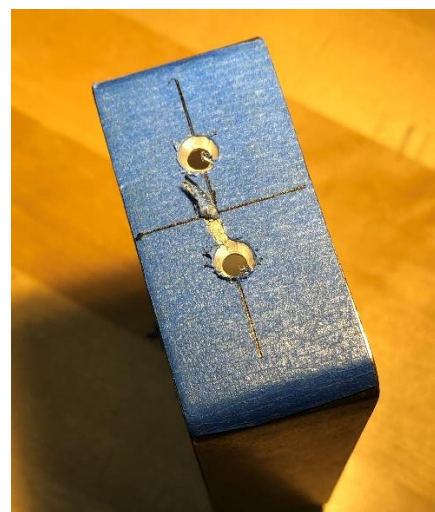
Counter sink added to the resistor mounting holes Figure 5
