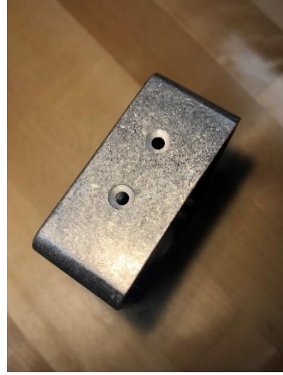
Flange resistor counter sink mounting holes Figure 7
